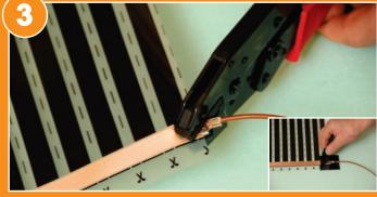
Connect the wiring harness to the heating element with the supplied crimping tool and insulate the connector with mastic adhesive tape.
