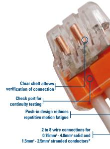
In-Sure<sup>®</sup> push-in wire connectors reduce installation time by up to 50%. They are the perfect replacement for traditional terminal blocks. The popular 2, 3 & 4 port models are rated to 32 Amps.
